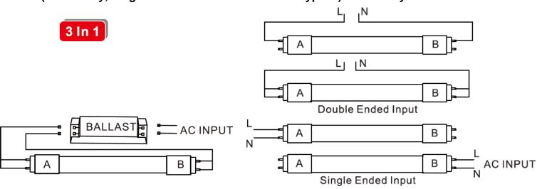
Ballast Compatible Input voltage: 120-277Vac 50/60Hz
